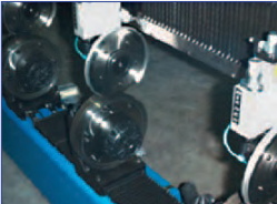
MAINTAINING SHEAR GEOMETRY: THE PNEUMATIC SHEAR KNIFE HOLDER
