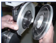
MAGNETIC BLADE REMOVAL TOOL
