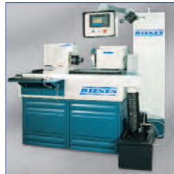
Dienes GR-1 automatic precision knife grinder
